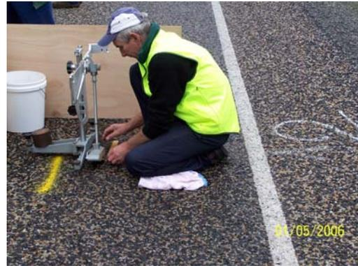
Figure 6. British Pendulum test on a 85/15 blend
