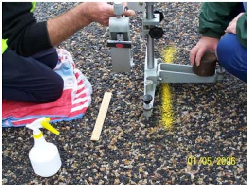
Figure 5. British Pendulum test on a 70/30 blend
