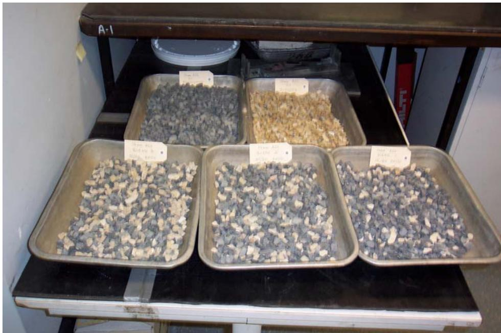
Figure 4. Blended products, basalt (control) and volcanic tuff.
