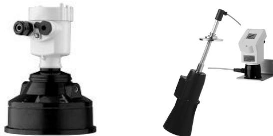
The transducer of the ultrasonic sensor transmits short high frequency ultrasonic pulses towards the product to be measured. The speed of the sound pulses is about 340m/sec. These pulses are reflected by the product surface and received again by the transducer as echoes. The running time of the ultrasonic pulses from emission to reception is proportional to the distance
